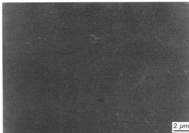
Figure 1 The result of scanning electron microscopy of the BaTiO 3 film on Si grown at 370 °C.
